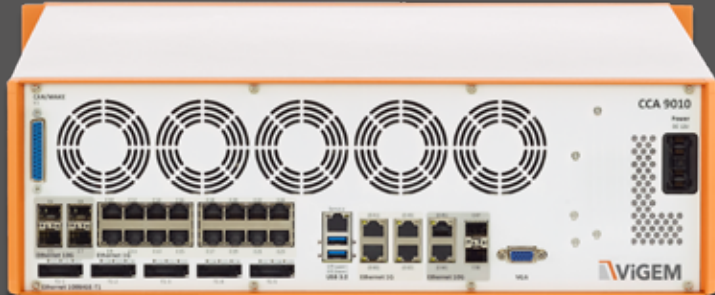
Rear side of the mid-range model CCA 9010-50: Continuous data recording up to 10 Gbit/s.
