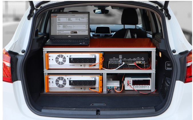
Img 1: ViGEM data logger CCA 9010 installed in the trunk of a vehicle.
